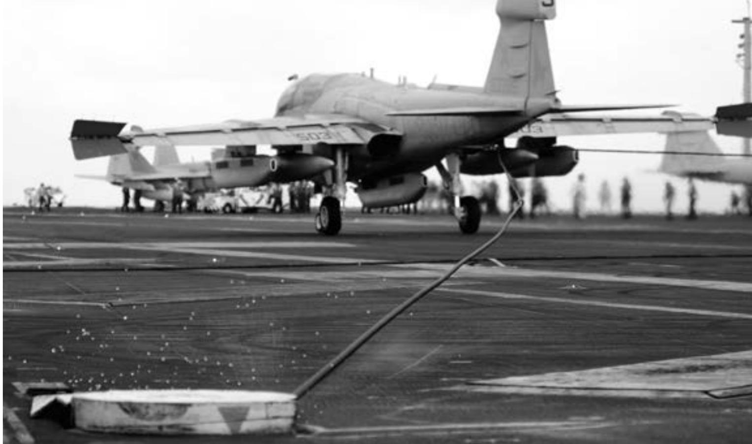
An EA-6B Prowler catches one of four arresting wires on the flight deck of an aircraft carrier.
